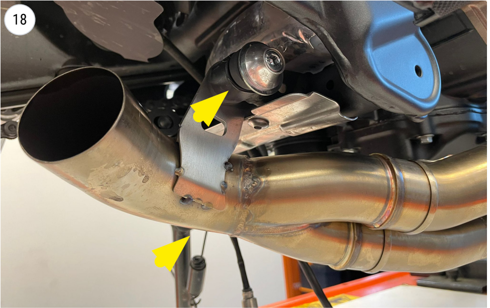
fit the pipe and screw
