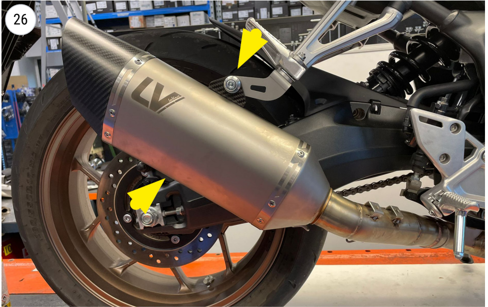
fit the muffler and screw
