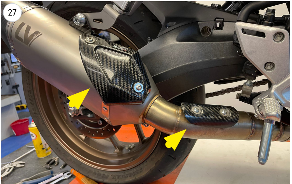
install the carbon heat shields
