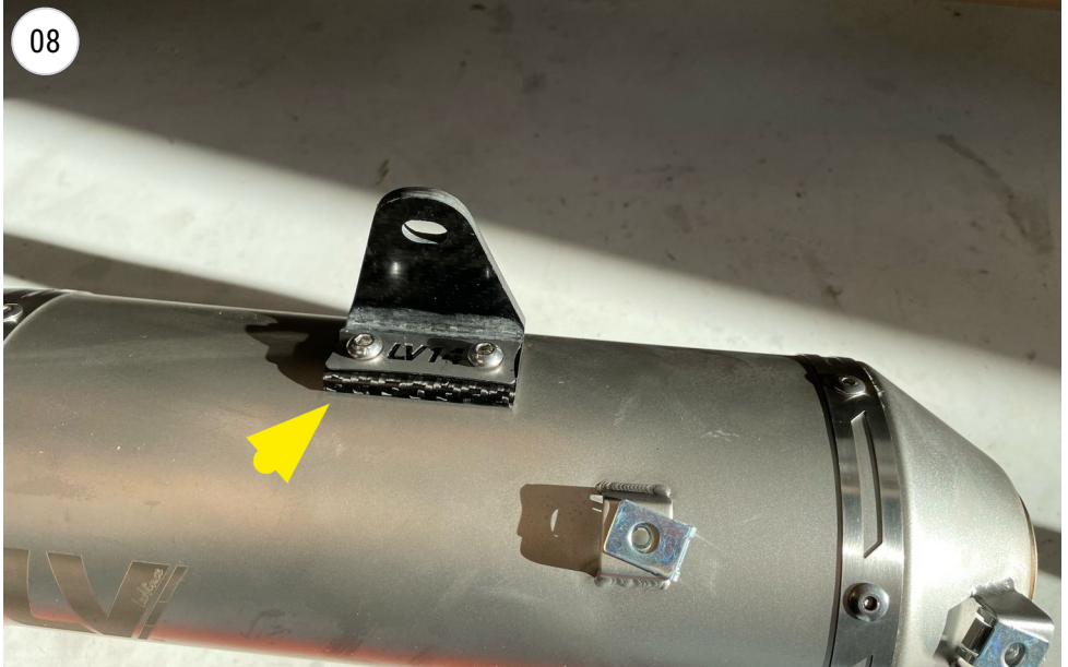
Screw on the carbon bracket with its plate without fully tightening the screws to allow for possible adjustments.
