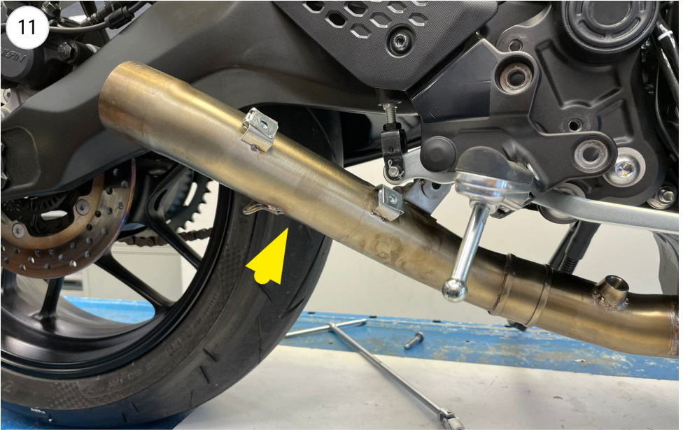
fit the final pipe
