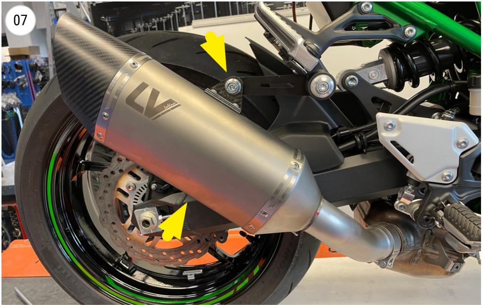
install the muffer
