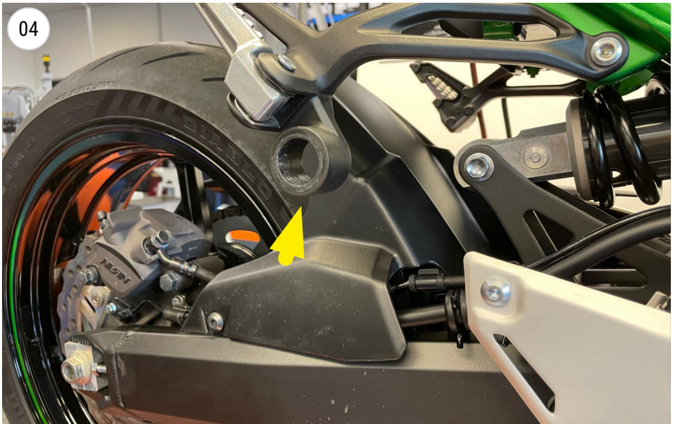
remove the stock spacers
