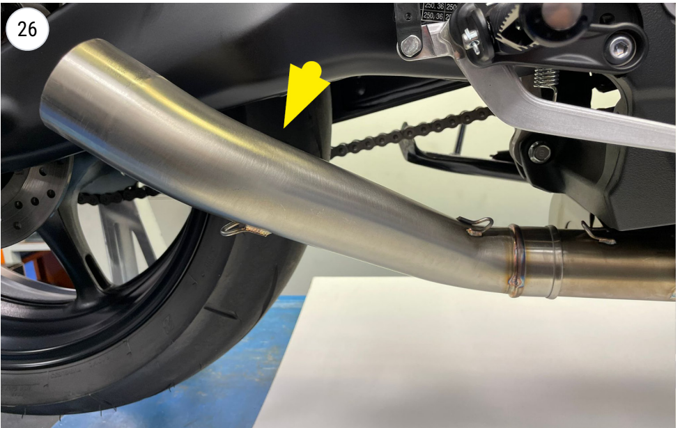
fit the final pipe
