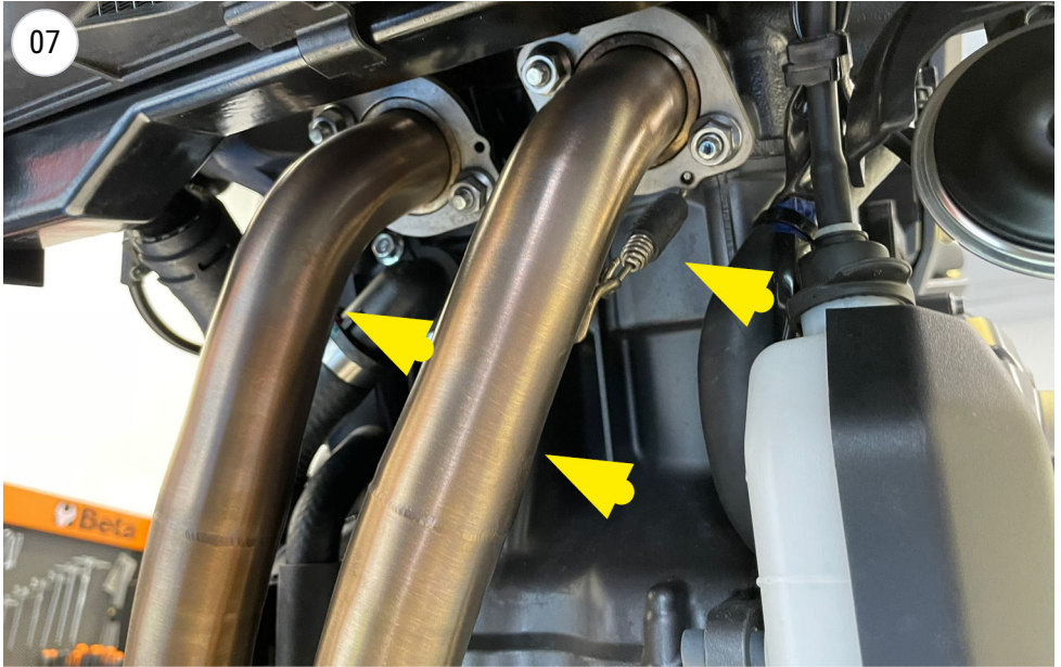
fit the primary pipes
