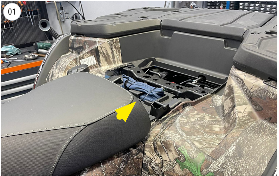
remove the passenger's seat
