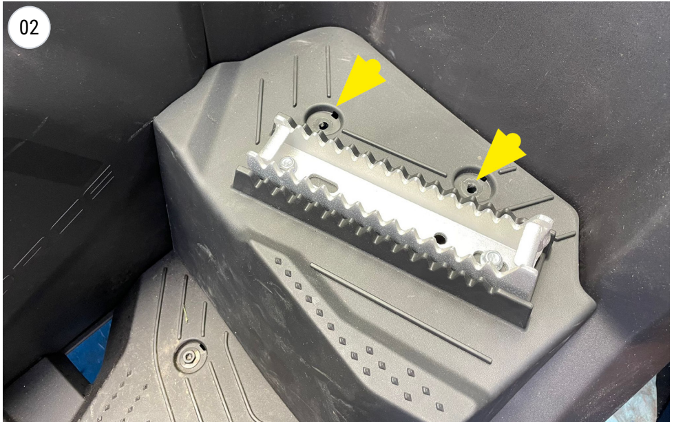
unscrew and remove the fairing
