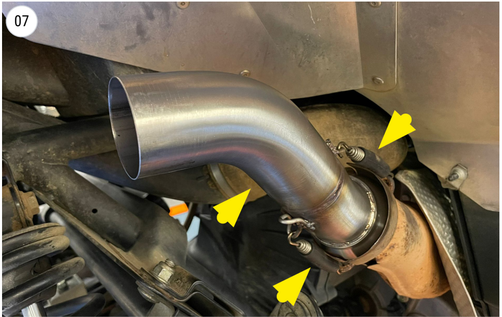
fit the pipe and hang the springs
