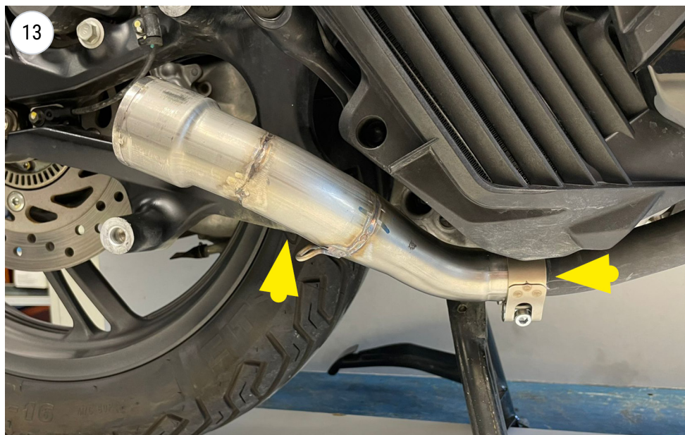
fit the pipe
