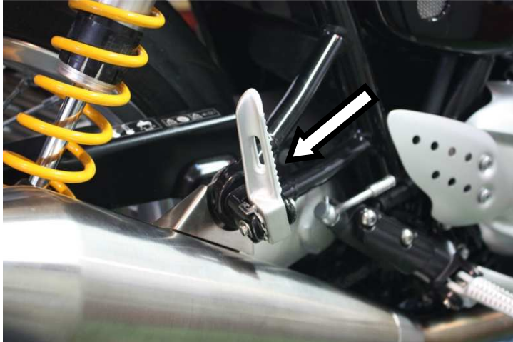
Smontare i pedalini dalle pedane passeggero DX ed SX Remove the footrest from LH and RH footpegs
